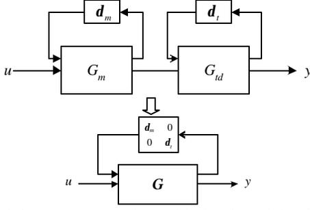
Fig. 3 System connection with the time delay block
