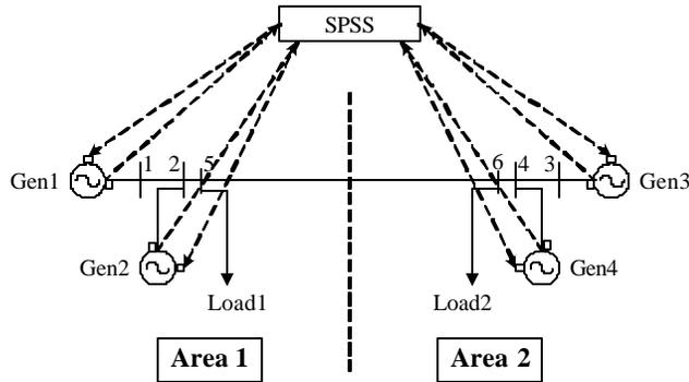
Fig. 6 A four-machine system with SPSS
