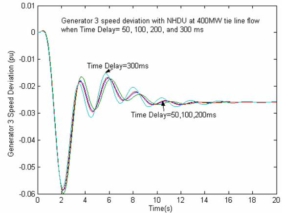
Fig. 10 Step response of Generator 3 speed deviation with NHDU for different time delays
