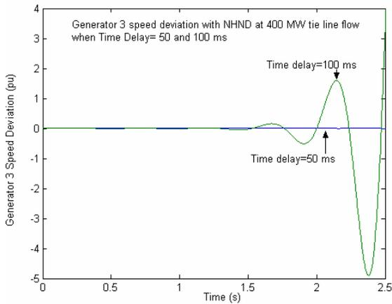
Fig. 9 Step response of Generator 3 speed deviation with NHND for different time delays
