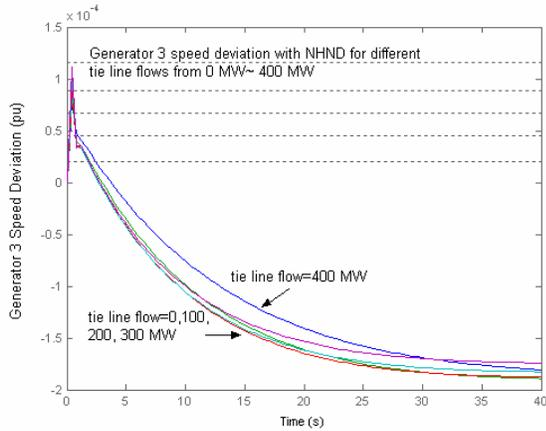
Fig. 8 Step response of Generator 3 speed deviation with NHND for different tie line flows
