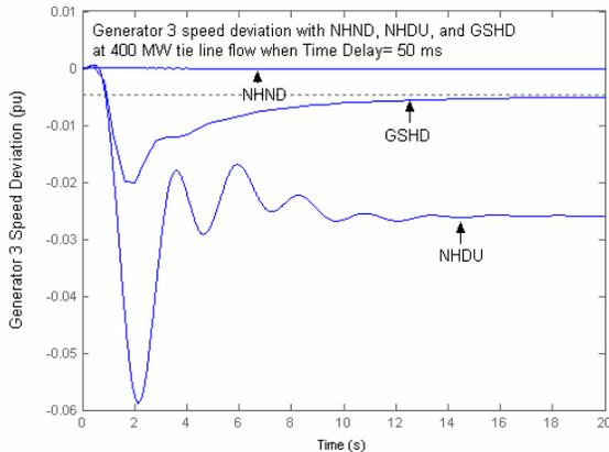
Fig. 12 Comparisons of the system performance with three controllers for a 50 ms time delay
