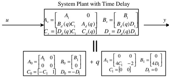
Fig. 5 System connection and the parameter-dependent form
