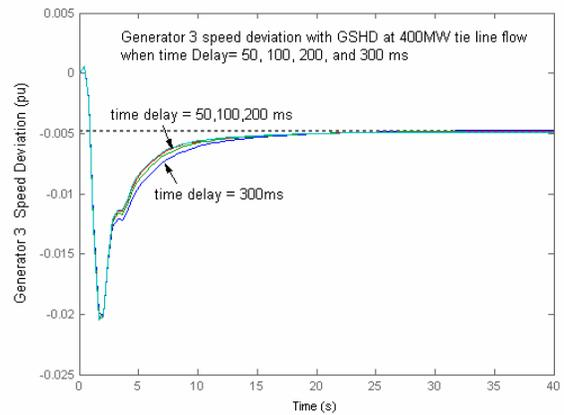
Fig. 11 Step response of Generator 3 speed deviation with GSHD for different time delays
