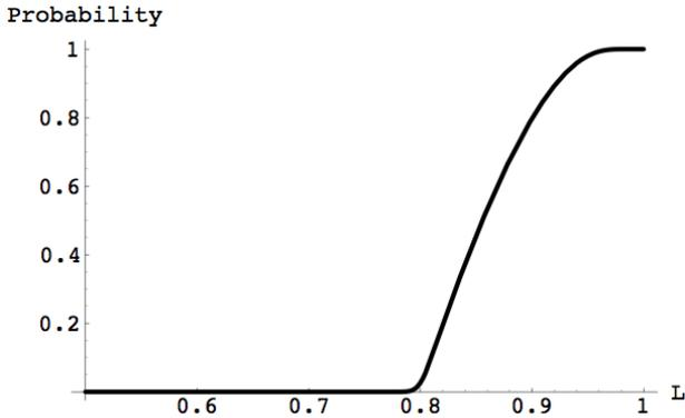
**Figure 8:** Probability of more than 500 components failed as a function of loading  $L$  in CASCADE model. There is a sharp increase at the critical loading  $L=0.8$ .
