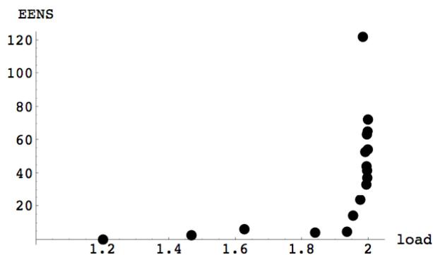
**Figure 2:** Expected energy not served as a function of the loading factor with respect to the base case. There is a sharp increase in blackout size at the critical loading of 1.94 times the base case loading.
