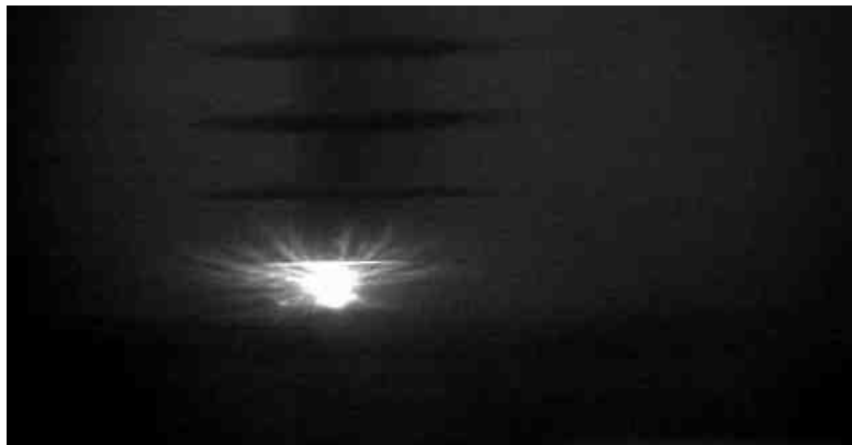
Figure 10: Discharge on a silicone rubber type nonceramic insulator at 80 KV
