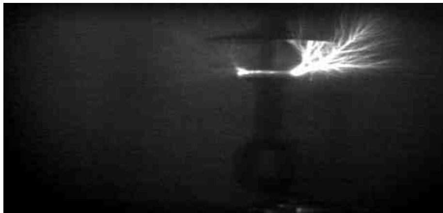
Figure 4: Corona at 80 KV of discharge magnitude 3.0 nC
