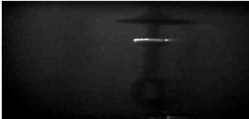
Figure 3: Corona at 50 KV of discharge magnitude 30 pC
