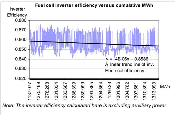
Figure 3.4: Fuel cell inverter efficiency versus cumulative MWh
