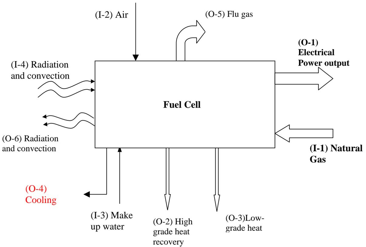
Figure 3.1: Input/output heat flows for the energy/mass balance
