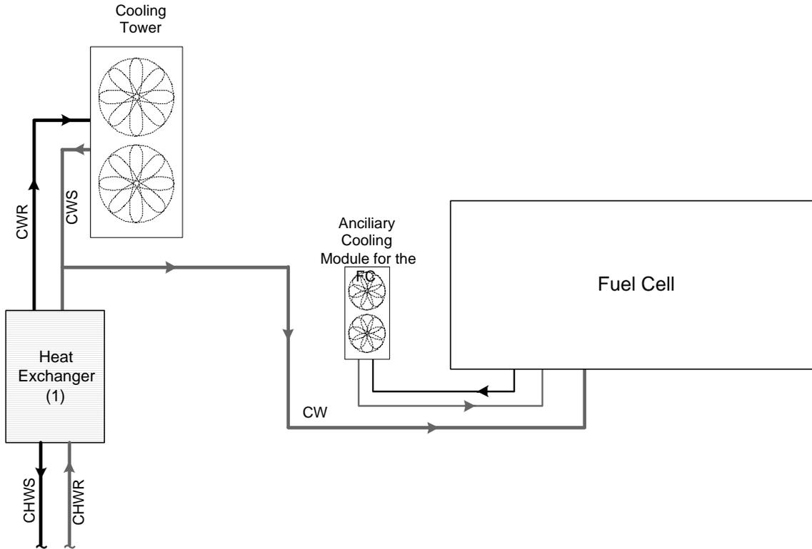
Figure 4.2: Ancillary cooling and makeup feed water arrangement
