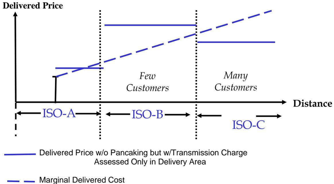
**Figure 2. Comparison of Delivered Cost of Electricity Including Recovery of Transmission Capital Costs**
